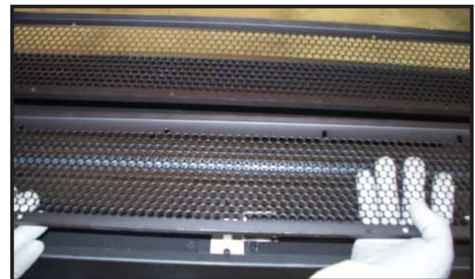
Figure 12.10 Lifting Base Pan Up and Out.
